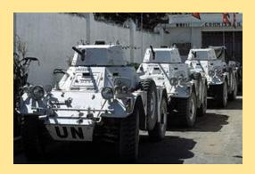
The Ferret scout car, is a British armoured fighting vehicle designed and built for reconnaissance purposes. The Ferret was produced between 1952 and 1971 by the UK company Daimler. It was widely adopted by regiments in the British Army, as well as the RAF Regiment and Commonwealth countries throughout the period.
